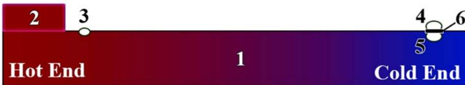
Fig. 2) 1 – Sample, 2 – heater, 3 – hot contact, 4 and 5 - contacts at the cold end, 6 - electrical insulator.
