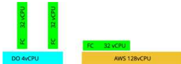
Fig. 1. System architecture for allowing live migration. Digital Ocean droplets and Amazon AWS ec2 instances are used as distinct public cloud entities. Firecracker provides a unified hypervisor on top and the orchestrator developed as part of this project monitors, snapshots, migrates virtual machines between DO and AWS hosts.
