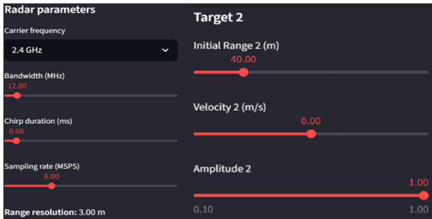
Figure 1. FMCW radar modeling interface implemented in Python.
